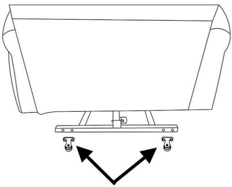
The supports will be found in the red hardware pack attached to the drive tube of the mechanism. Please follow the steps listed in the assembly instructions for proper attachment.
