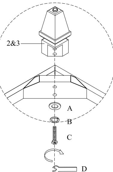
DO NOT TIGHTEN BOLTS UNTIL THE UNIT IS COHMPLETELY ASSEMBLED.
