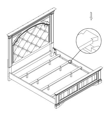
Step 5: Attach the assembly slat with middle leg into the groove on the side rail. assembly product is now completed.
