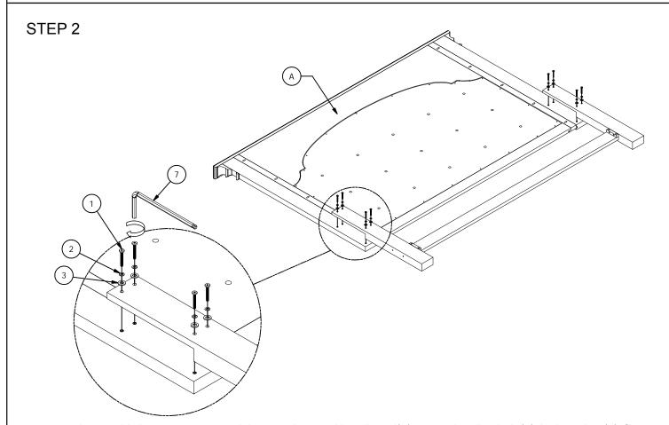
Step 2: Attach assembly bottom support with leg into the panel headboard(A). insert the allen bolt (1), lock washer (2), flat washer (3) into the hole, tighten with allen key(7)
