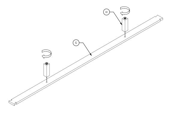
Step 4: Assemble the middle leg (H) with slat (G). tighten at this time.
