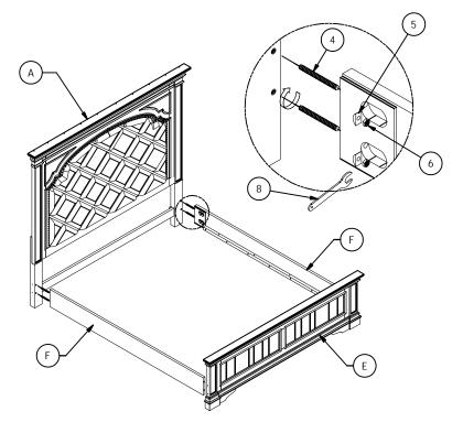
Step 3: Insert the long drat (4) into the assembly headboard (A) and footboard (E), tighten all long drat at this time. Then assemble side rail to headboard and footboard using halfmoon (5), hex nut (6) as picture shown, tighten with wrench(8)
