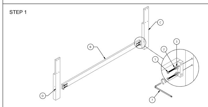
Step 1: Place all parts down on a piece of cloth or carpet to prevent finish from scratching. insert allen bolt (1), lock washer (2), flat washer (3) into the hole to the bottom support (B) and then assemble with leg (C) & (D). tighten with allen key (7)
