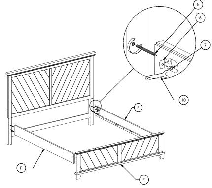
Step 3: Insert the long drat (5) into the assembly headboard and footboard (E), tighten all long drat at this time. Then assemble side rail to headboard and footboard using halfmoon (6) and hex nut (7) as picture shown, tighten with wrench(10)
