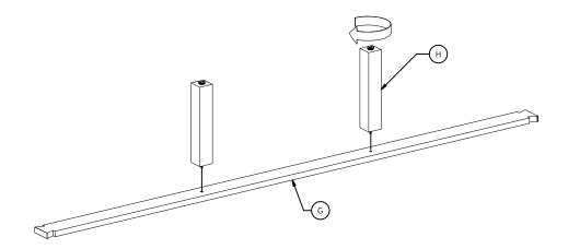
Step 4: Assemble the middle leg (H) with slat (G). tighten at this time.
