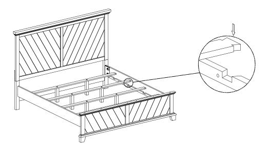
Step 5: Attach the assembly slat with middle leg into the groove on the side rail. Assembly product is now completed.
