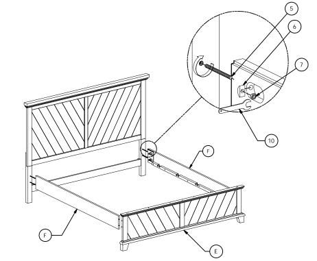
Step 3: Insert the long drat (5) into the assembly headboard and footboard (E), tighten all long drat at this time. Then assemble side rail to headboard and footboard using halfmoon (6) and hex nut (7) as picture shown, tighten with wrench(10)
