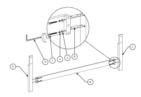
Step 1: Place all parts down on a piece of cloth or carpet to prevent finish from scratching. insert the wood dowel (8) to the bottom support (B) and then assemble with leg (C) & (D). insert allen bolt (1), lock washer (4), flat washer (3) into the hole. tighten with allen key (9)
