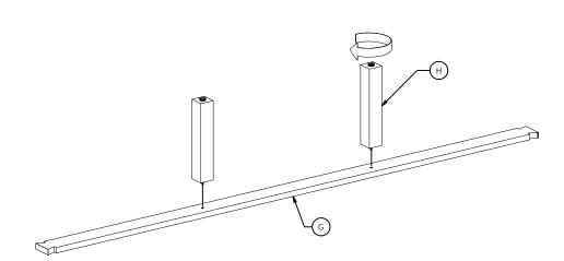
Step 4: Assemble the middle leg (H) with slat (G). tighten at this time.
