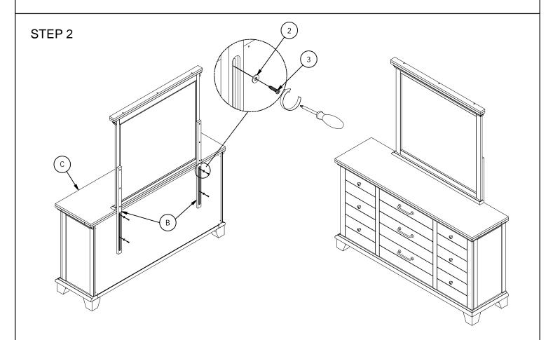
Step 2: Attach connecting bar (B) to drawer dresser (C). insert the screw (3), flat washer (2) into the groove on the connecting bar(B), tighten with screwdriver (not provided). Assembly product is now completed.
