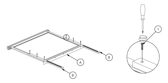
Step 1: Place all parts down on a piece of cloth or carpet to prevent finish from scratching. insert the screw (1) in to the hole on the connecting bar (B) and then assemble with mirror (A), tighten with screwdriver (not provided).
