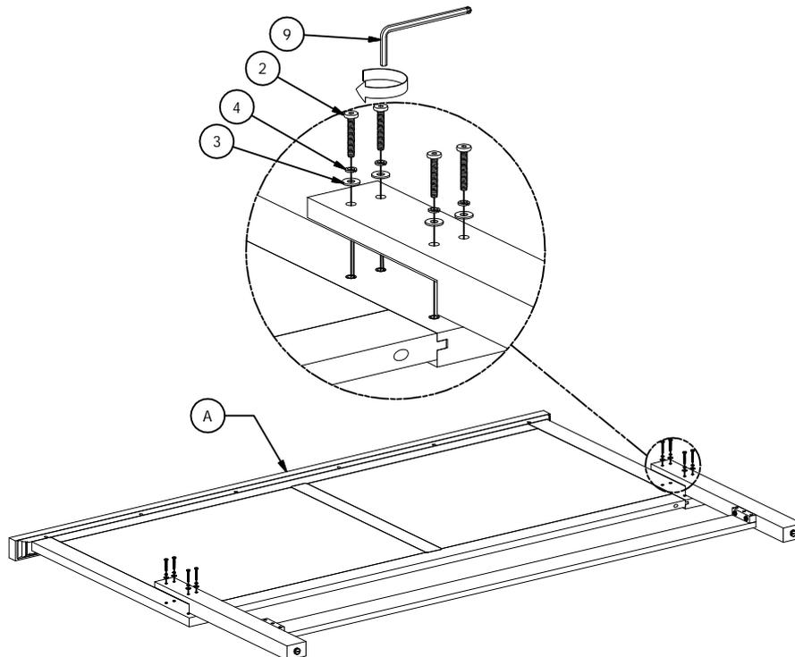
Step 2: Attach assembly bottom support with leg into the panel headboard(A). insert the allen bolt (2), lock washer (4), flat washer (3) into the hole, tighten with allen key (9)
