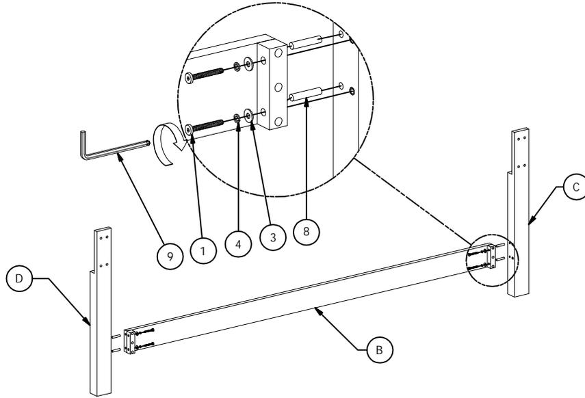
Step 1: Place all parts down on a piece of cloth or carpet to prevent finish from scratching. insert the wood dowel (8) to the bottom support (B) and then assemble with leg (C) & (D). insert allen bolt (1), lock washer (4), flat washer (3) into the hole. tighten with allen key (9)
