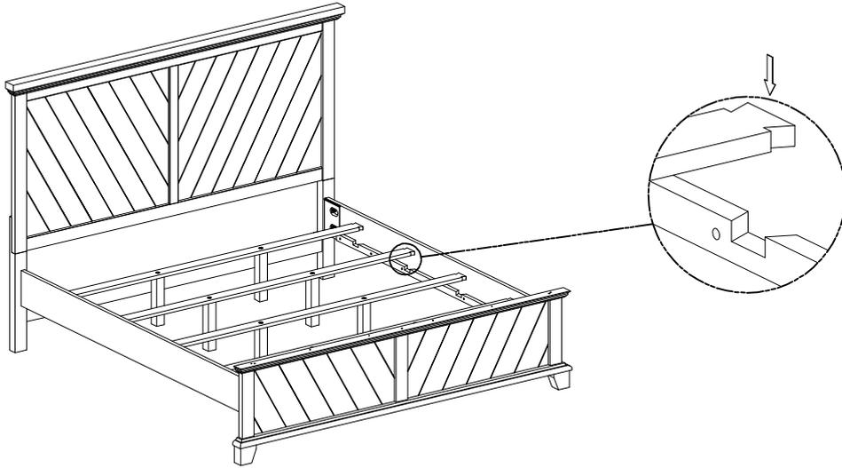
Step 5: Attach the assembly slat with middle leg into the groove on the side rail. Product assembly is now completed.
